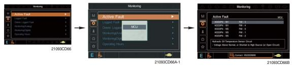
$\cdot\,$  The active faults of the MCU can be checked by this menu.
