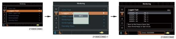
$\cdot\,$  The logged faults of the MCU can be checked by this menu.
