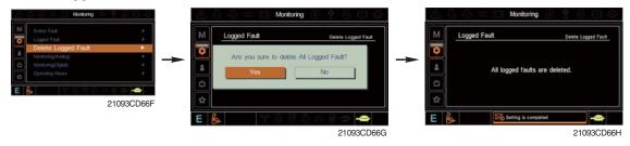
$\cdot\,$  The logged faults of the MCU can be deleted by this menu.
